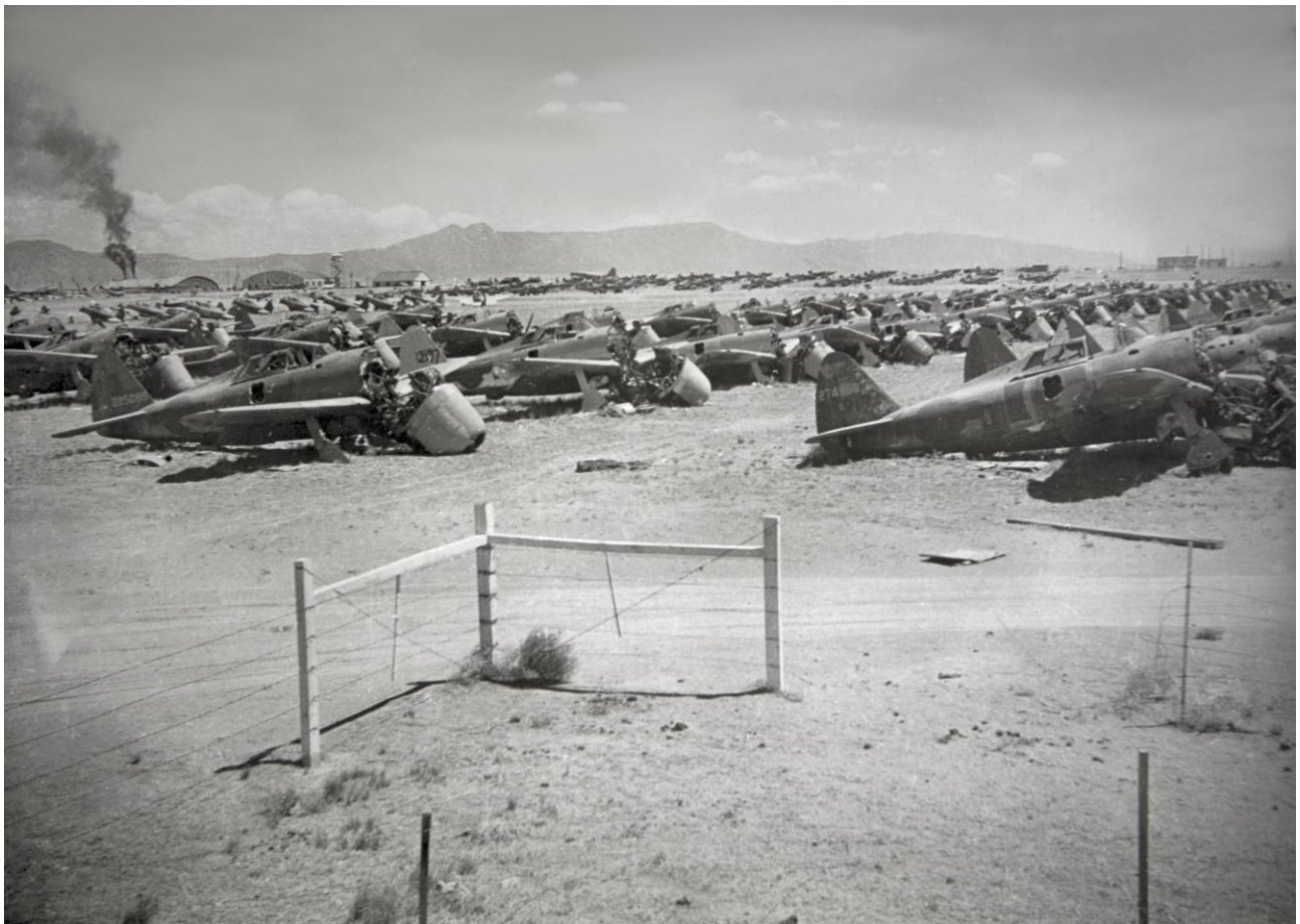
Early razorback P-47 fighters being striped down for disposal. The smoke in the background is the smelter used to melt the planes into ingots of aluminum. The
