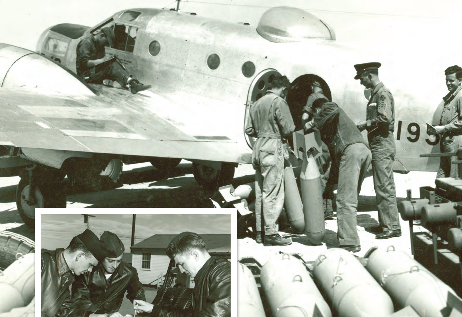
Training bombs (Above) are loaded onto an AT-11. The bay held ten 100-lb practice bombs. These inert bombs were filled with sand. A black powder charge exploded when the bomb hit the ground, allowing its target accuracy to be judged by the in-flight instructor. Cadets (Left) work out a navigation problem prior to their practice bombing mission. (Both Images Courtesy Air Force Nuclear Weapons Center Office of History)
