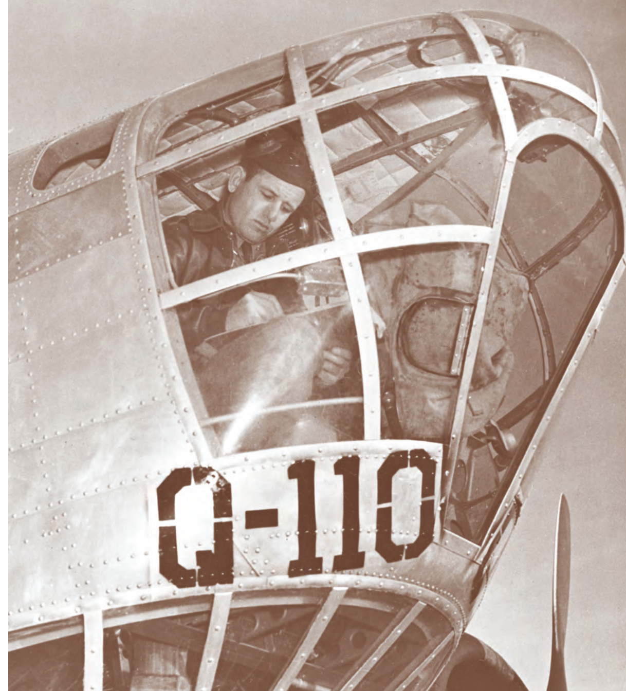
The bombardier's section of the aircraft was sometimes called "the greenhouse" due to its appearance. This student bombardier at Kirtland Field sits in the greenhouse of a Douglas B-18 Bo/o . Visible below it is the nose gunner's station. (Courtesy Air Force Nuclear Weapons Center Office of History)
